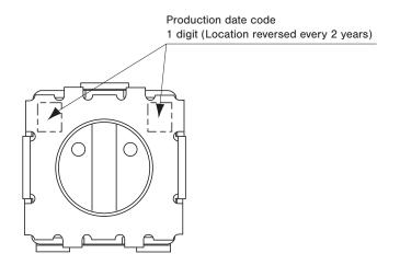
The model that this marking method is applicable: Rotary switch CS-32
