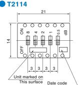
Unless otherwise specified, tolerance :  $\pm$  0.3 (Unit : mm)
