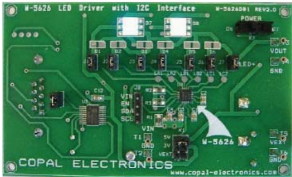
Figure 2. W-5626DB1 Component Placement – Top Side
