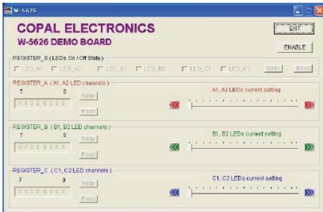
Figure 3. W-5626DB1 Software Interface Window (start window)
