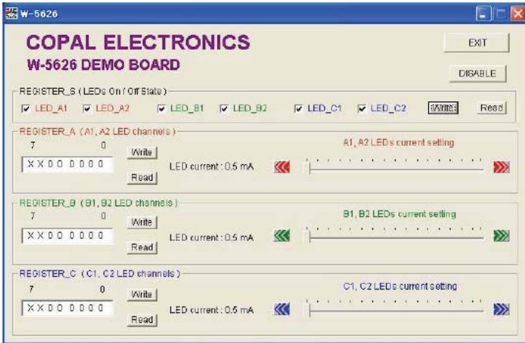
Figure 4. W-5626DB1 with all channels enabled and LED currents set to min value
