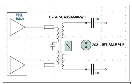
The diagram above shows protection in an application, but does not constitute a complete circuit design.
