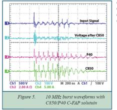
Channel 1: 10 MHz burst generator voltage surge Channel 2: Clamp diodes between C850 and input to P40 Channel 3: Let-through current of P40 Channel 4: Let-through current of C850
